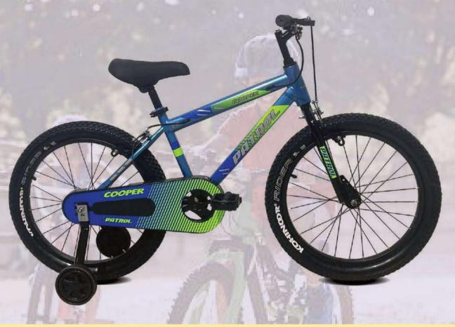
FRAME: HI-TENSILE STEEL FRAME WITH INTERNAL CABLE, FORK: RIGID FORK, BRAKES: F/R CALIPER BRAKES, TIRE: 20 X 2.40 COTTON, RIM: SINGLE WALL STEEL, ADD ON: TRAINER WHEELS
